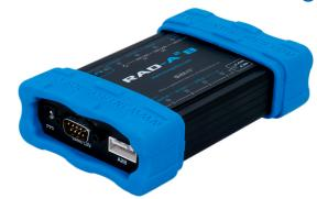
RAD-A2B combines Analog Devices' A2B technology with two CAN/CAN-FD transceivers and one LIN channel to allow mixed network messages in one time stamped log. The RAD-A2B tool includes one channel for A2B receive-only monitoring and one channel that can act as an emulator node.
